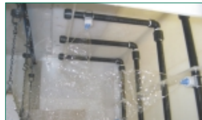
Low pressure flowcoat in operation (above) and close-up of baffles designed to control air flow (right).
