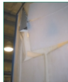
Low pressure flowcoat in operation (above) and close-up of baffles designed to control air flow (right).
